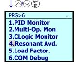
7. Using the key to move the cursor to Fjmp3 and pressing the key at the next point of resonance sets resonance prevention point 3 (Fjmp3).
