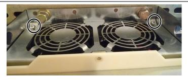
(3) Turn the fan casing in the direction of the arrow and pull it towards you.
