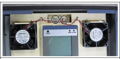
(2) Pull the latches securing the fans in the direction of the arrows and remove the fans.
