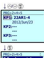
5. Use the ⊘/ ⊗ keys to select the location, KP1–KP3, to store the data to be confirmed, and confirm the destination with the ⊯ key.
