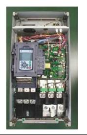
Disconnect the three fan power connectors marked with ellipses.
