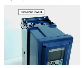
Remove the cooling fan (with case).
