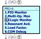
3. Use the ⊘/ ⊗ keys to select [3. CLOGIC Monitor], and confirm with the (♣) key.
