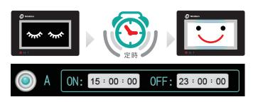
Users can set the screen turn on/off time from HMI system menu "Power Setup\Auto Stand by Wakeup Setting". HMI turns off screen when it goes into power save mode. The maximum number of setting items is 8.
