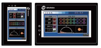
EC205-CT0A model add a function which is ertical / horizontal display. The designer can adjust the display direction easily by panel size or user's demand.
