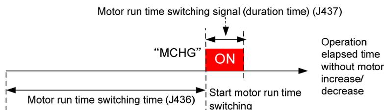
Furthermore, the motors in which forced on (forced commercial power drive) (J411 to J414 = 2) is selected in motor mode selection shall not be subject to motor operating time switching.
