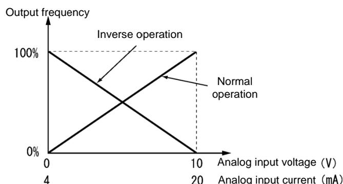
**Tip** The normal/inverse switching operation is useful for air-conditioners that require switching between cooling and heating. In cooling, the speed of the fan motor (output frequency of the inverter) is increased to lower the temperature. In heating, the speed of the fan motor (output frequency of the inverter) is reduced to lower the temperature. This switching is realized by the IVS.
