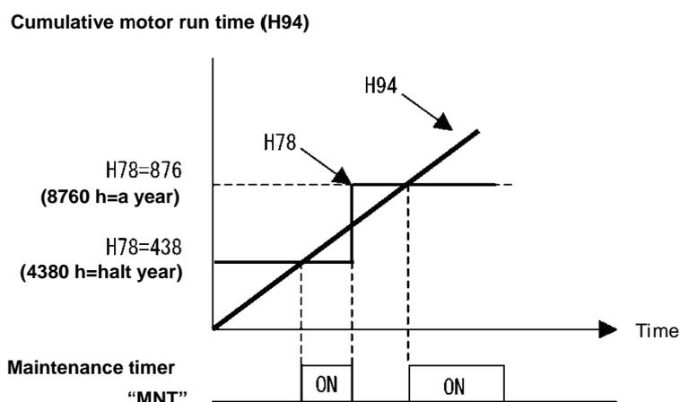
**Note** If the maintenance interval is reached, set a new value in H78 and press the
