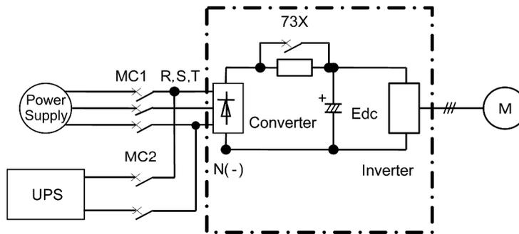
Figure J.9 Connection diagram example
