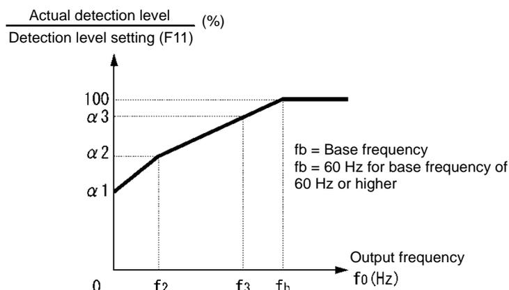
Figure J.5 Characteristics diagram of motor cooling system
