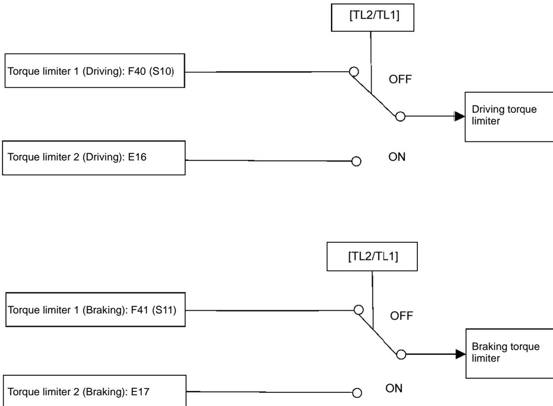
Figure J.8 Switching torque limits diagram
