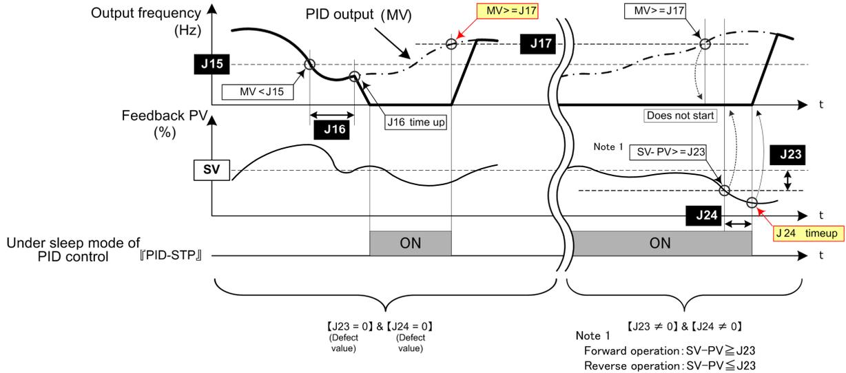
**J18, J19** PID Control (Upper limit of PID process output, Lower limit of PID process output)
