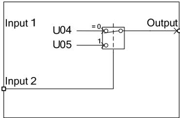
(4005) Low pass filter with enable
