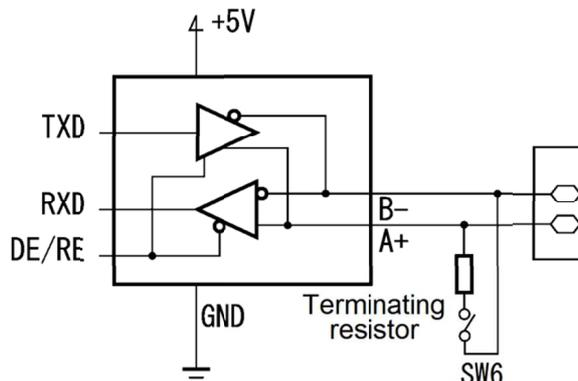
\* The terminating resistor 112 Ω is built in. Open/close with SW6. \*
