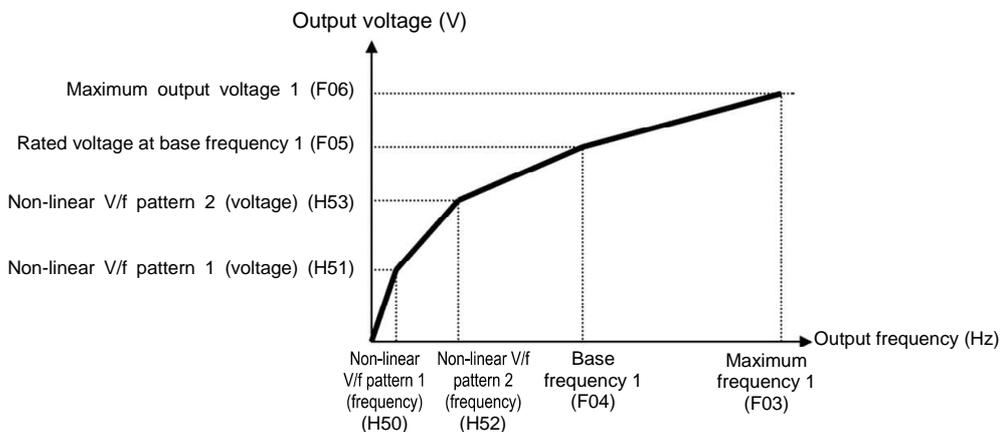
Figure J.4 Characteristics diagram of no-linear V/f pattern setting (2 points)
