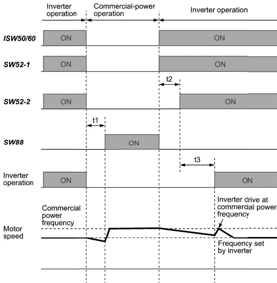
t1: 0.2 sec + Time specified by H13 (Restart mode after momentary power failure)
