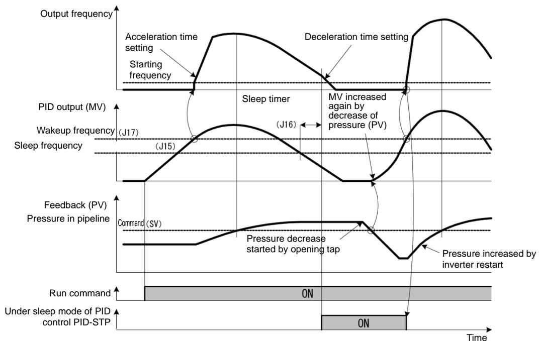
■ PID control (Wakeup level of PID error) (J23)
