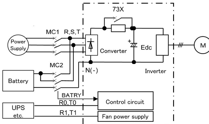
Figure J.12 Connection diagram example (FRN0203E2■-4EH or above)
