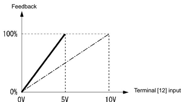
**PID display coefficient and Monitoring**
