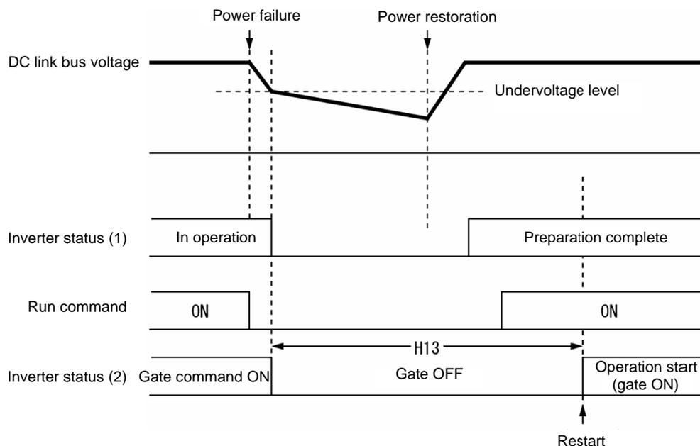
Factory default: At the factory default state, setting is performed so that it is appropriate to the standard motor (refer to "1.3 Factory default value per applicable electric motor capacitance"). Basically, there is no need to modify the default setting. However, when problems occur due to the long holding time or decrease in flow rate of pump becomes significant, change to about half of the standard value and make sure that alarm etc. will not occur.
