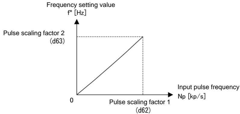
Figure J.2 Relationship between input pulse frequency and frequency setting value
