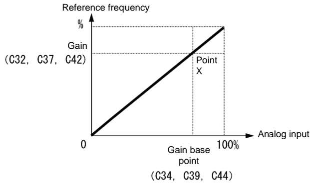
**Note** To input bipolar analog voltage (0 to ±10 VDC) to terminal [12], set C35 data to “0.” Setting C35 data to “1” enables only the voltage range from 0 to +10 VDC and interprets the negative polarity input from 0 to -10 VDC as 0 V.
