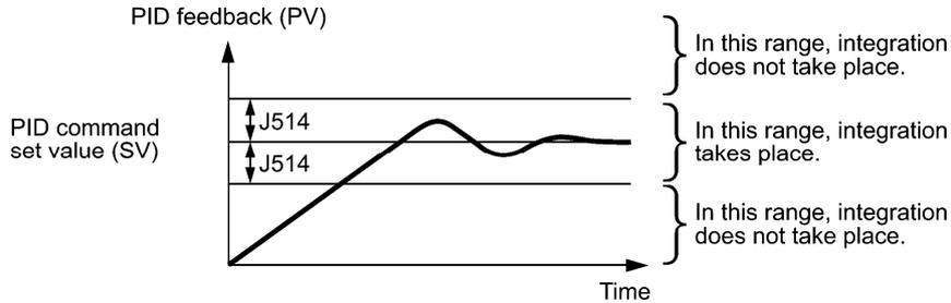
**J515 External PID Control 1 (ON/OFF control hysteresis width)**
