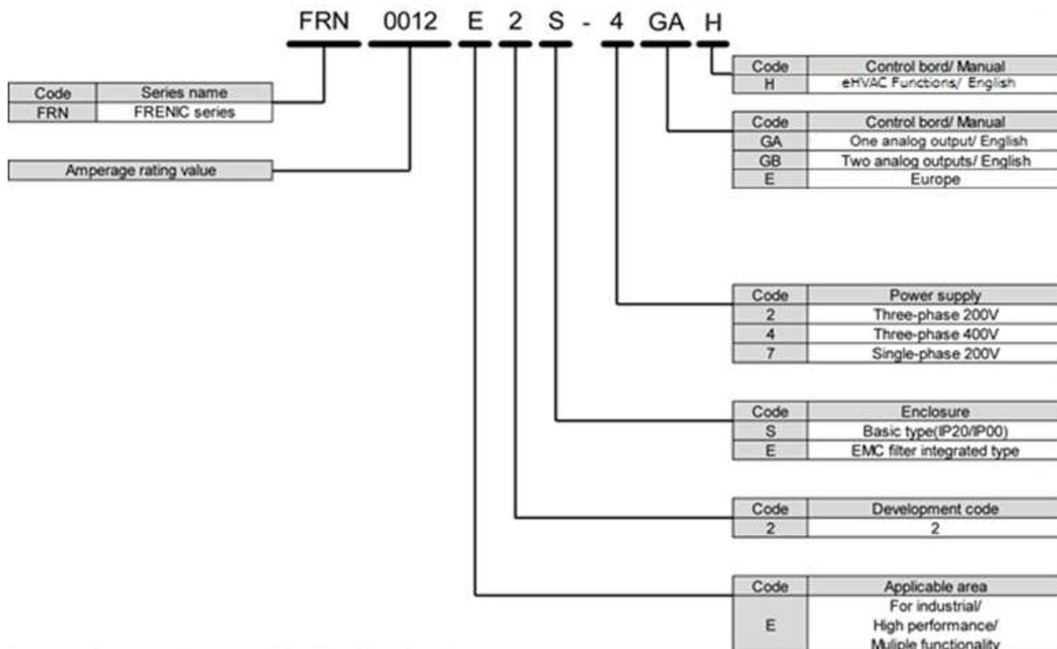
Figure H-2 Type of inverter
