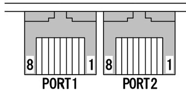
Figure M.12-1 Pin assignment
