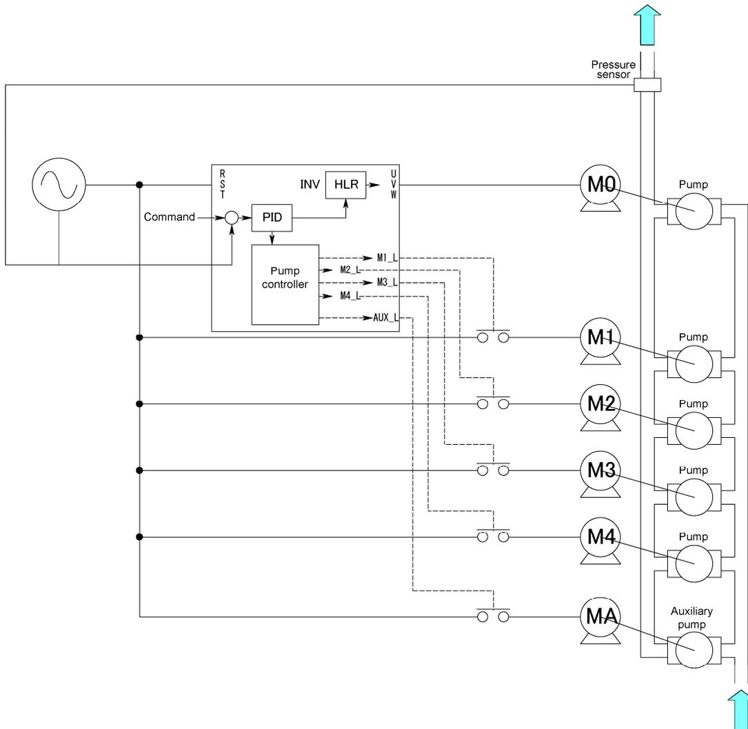
Figure J.24 Configuration diagram
