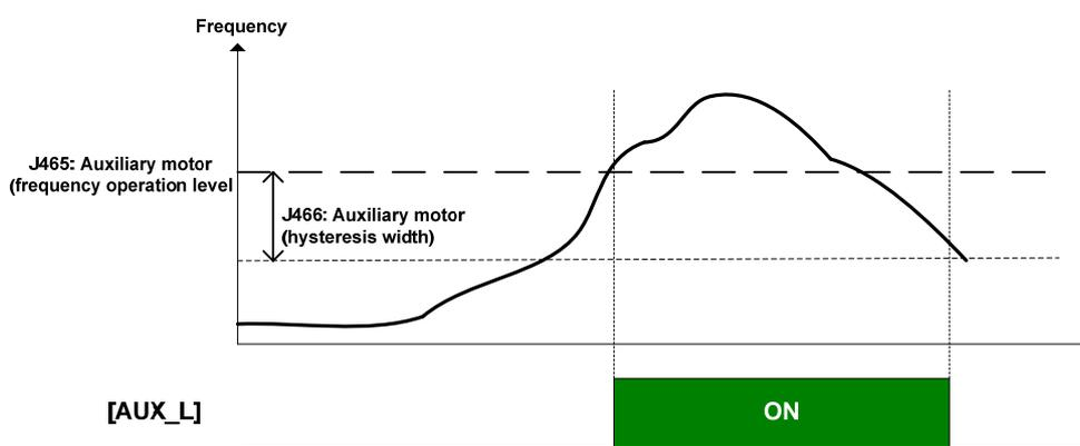
■ **Auxiliary motor (frequency operation level) (J465)**
