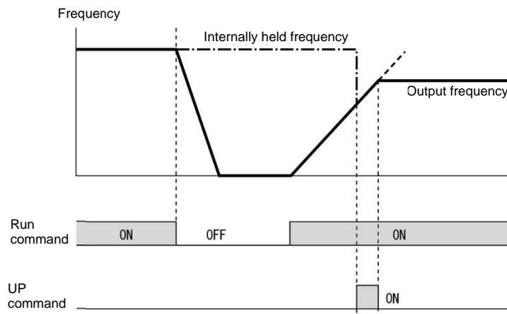
**[ 4 ] Frequency setting using digital inputs (option DIO interface card) (F01 = 11)**
