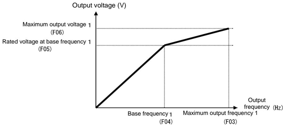
Figure J.3 Characteristics diagram of normal V/f pattern setting
