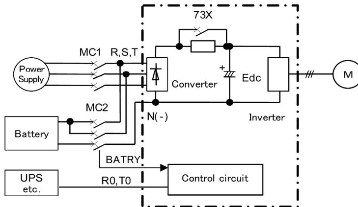
Figure J.11 Connection diagram example (FRN0020E2■-2G□H or below, FRN0168E2■-4EH or below)
