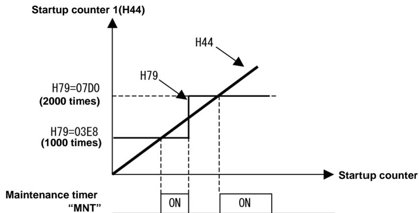
**Note** If the startup counter reaches the specified value, set a new value for the next maintenance in H79 and press the
