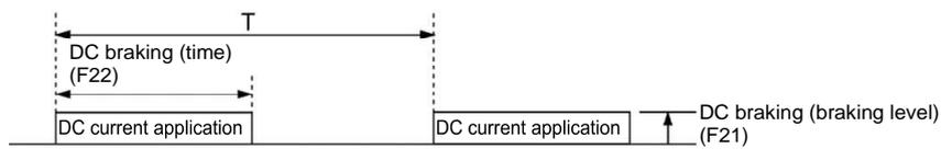
Figure J.23 Dew condensation prevention operation
