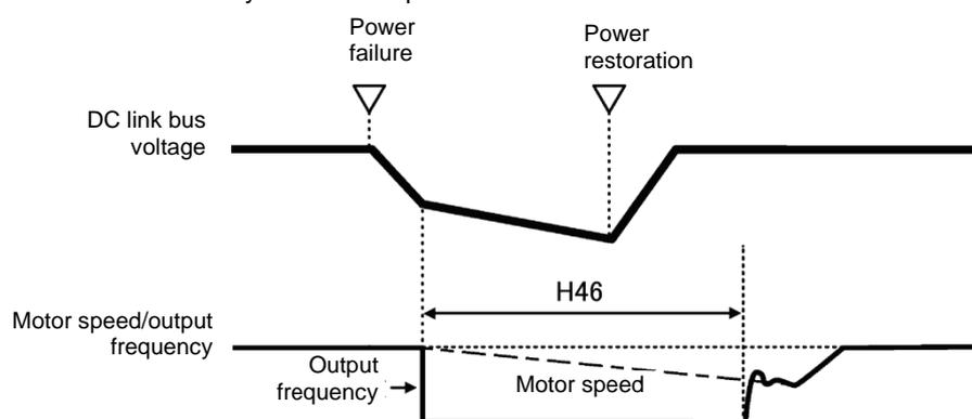
Under auto search control, the inverter searches the motor speed with the voltage applied at the motor start and the current flowing in the motor, based on the model built with the motor parameters. Therefore, the search is greatly influenced by the residual voltage in the motor.
