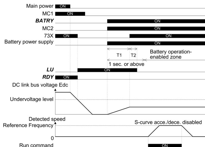
Figure J.J Battery operation timing chart
