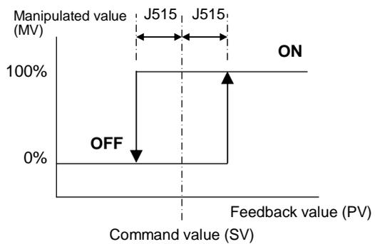
**J516 External PID Control 1 (Proportional operation output convergent value)**
