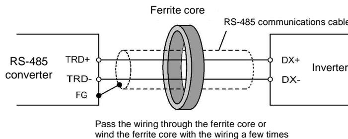
Figure K.5-1 Adding an Inductance Component
