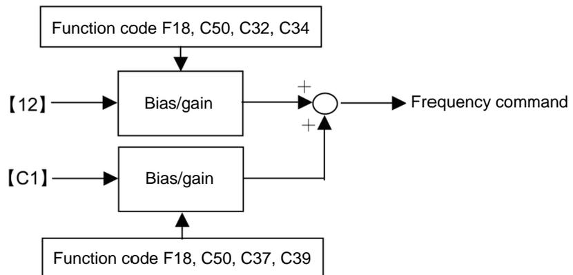
For single polarity (Terminal [12] (C35=1), Terminal [C1] (C1 function), Terminal [C1] (V2 function). As the above diagram indicates, for reference frequency and analog input of frequency setting 1, it is possible to set arbitrary relationship by A point (determined by bias (F18) and bias reference point (C50)) and B point (determined by the gain corresponding to each analog input and the gain reference point (C32 and C34, C37 and C39, and C42 and C44)).
