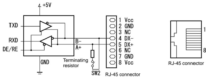
\* The terminating resistor 112 Ω is built in. Open/close with SW2. \*
