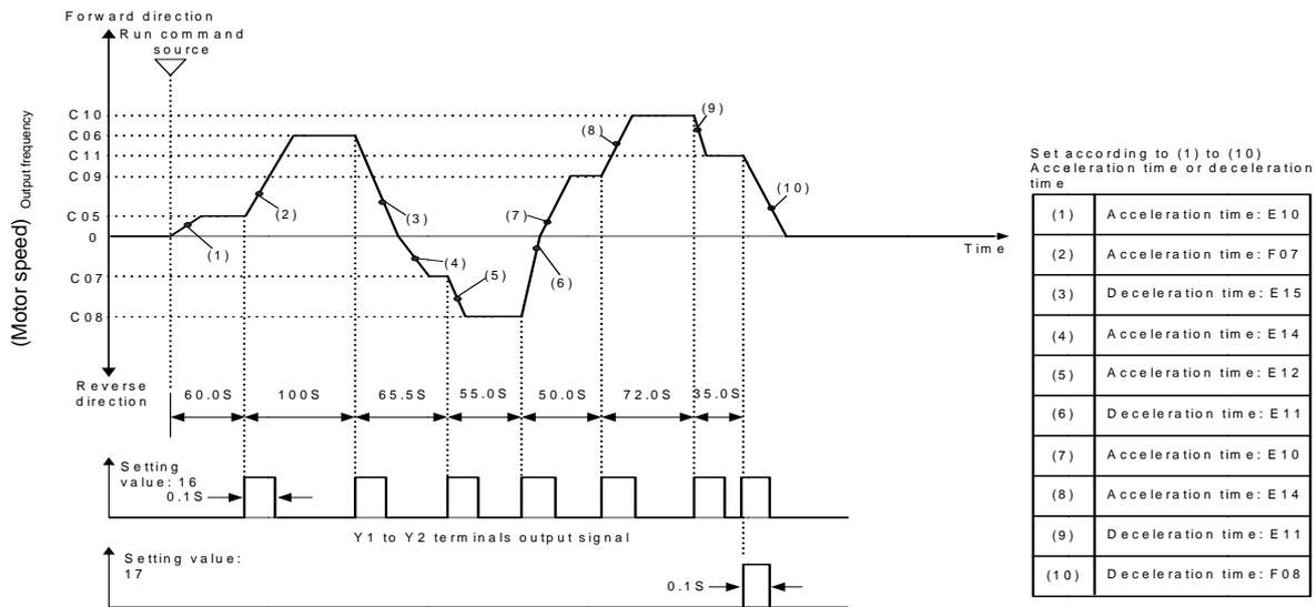
F08 Deceleration time 1 setting is used as deceleration time for deceleration to stop after the completion of one cycle.
