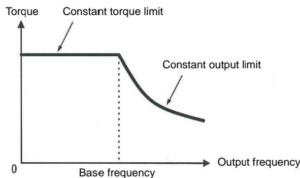
■ **Torque limiter (F40, F41, E16, E17) Data setting range: 0 to 300%; 999 (Disable)**
