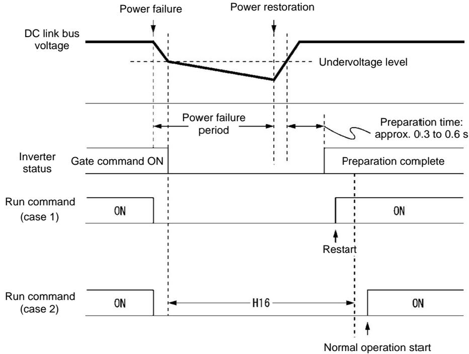
When allowable momentary power failure time (H16) is set to “999”, momentary power failure restart is performed until DC link bus voltage decreases by momentary power failure restart allowance voltage (100 V for 400 V class), however, if the voltage becomes at or below the momentary power failure allowance voltage, the state is judged as a power shut down. As a result, the inverter operates as powering ON again without performing momentary power failure restart operating.
