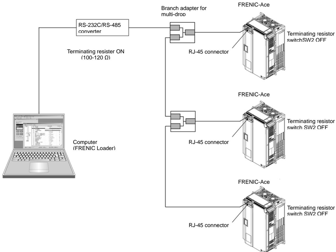
Figure K.3-1 Multi-drop Connection for RS-485 Communication Port 1 (Using the RJ-45 Connector)
