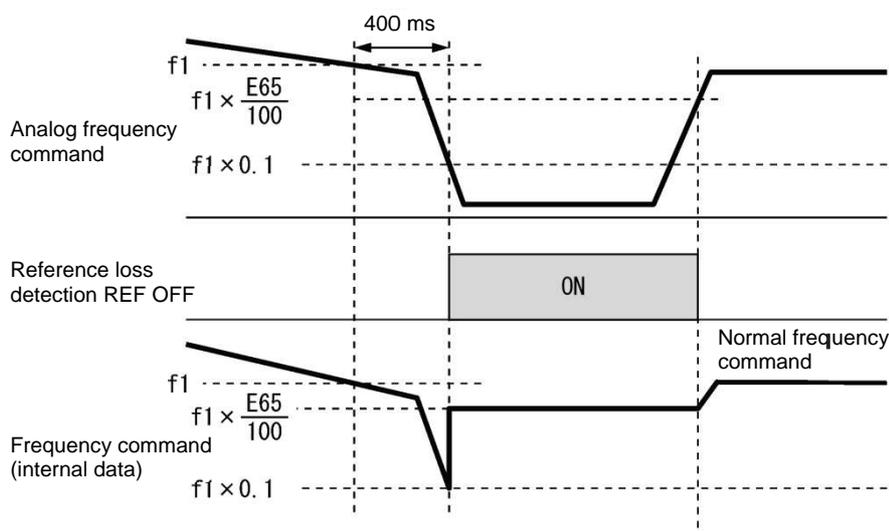
In the diagram above,  $f_1$  is the level of the analog frequency command sampled at any given time. The sampling is repeated at regular intervals to continually monitor the wiring connection of the analog frequency command.
