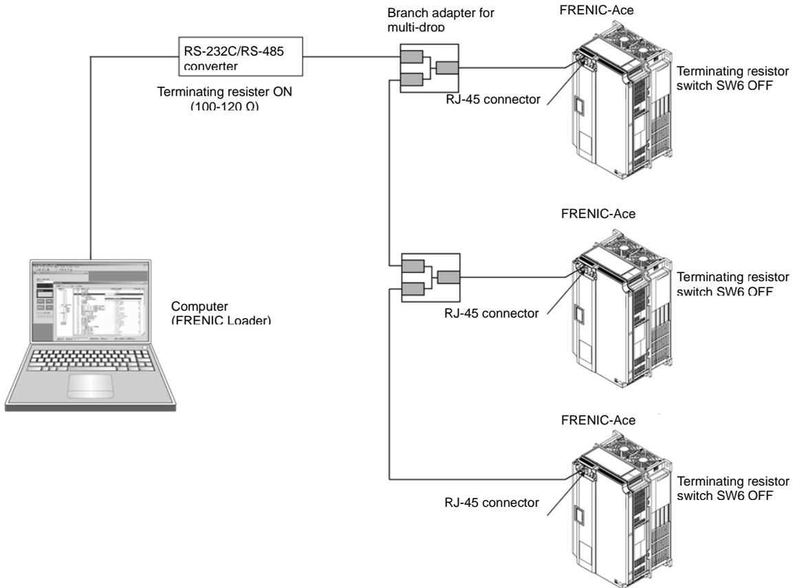
Figure K.3-2 Multi-drop Connection for RS-485 Communication Port 2 (Using the RJ-45 Connector)
