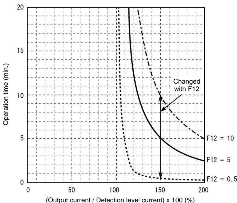
Figure J.6 Example of current-operation time characteristics
