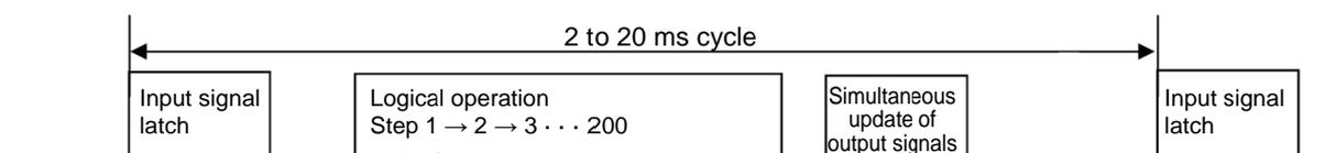
Note that if you do not consider the process order of customizable logic when configuring a function block, the expected output may not be obtained, the operation can be slower or a hazard signal can occur, because the output signal of a step is not available until the next cycle.
