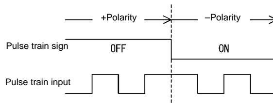
Figure J.1 Pulse train sign/Pulse train input.
