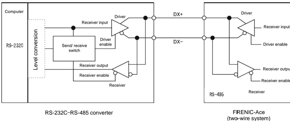
Figure K.4-1 Communication Level Conversion
