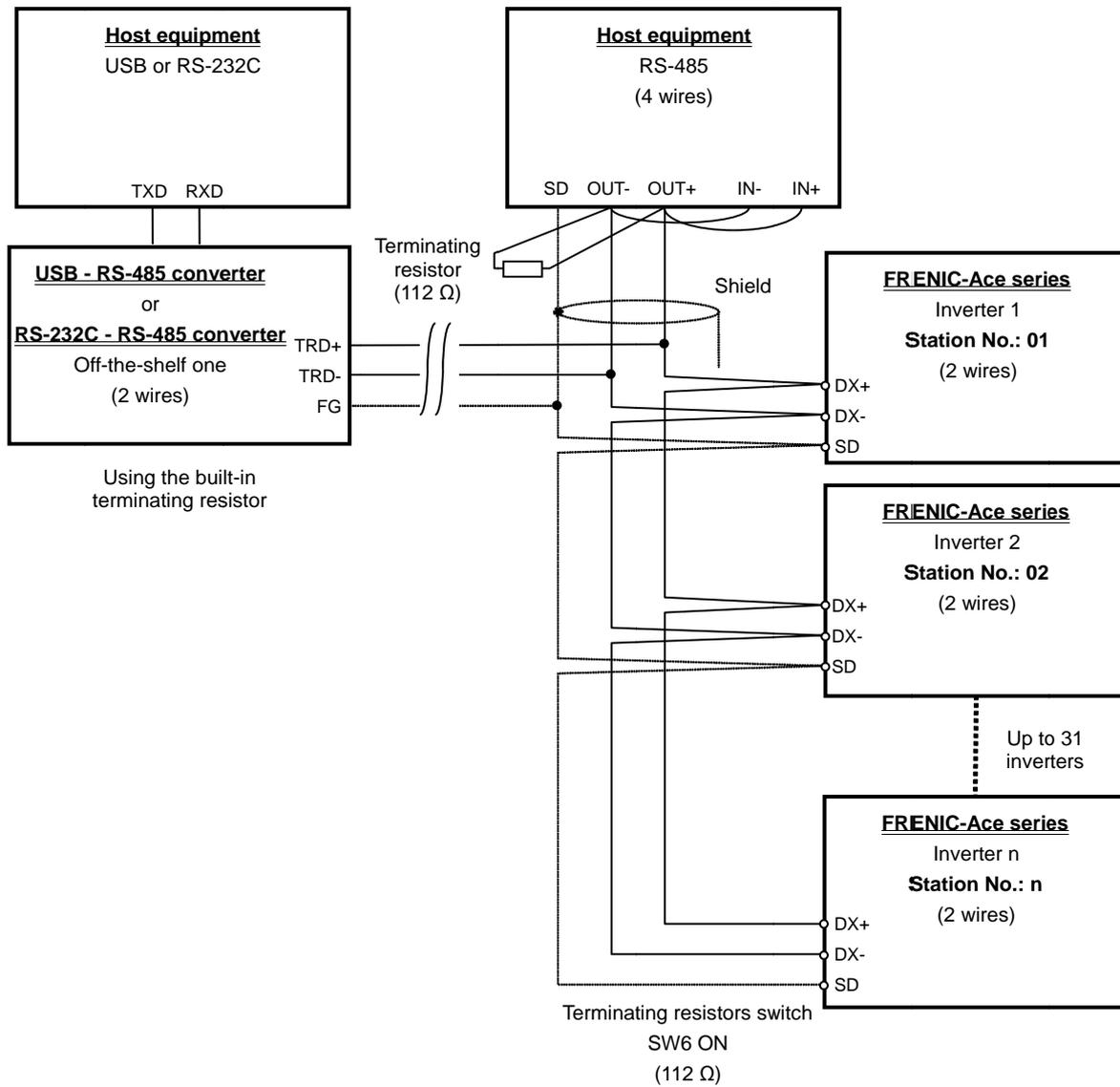
Figure K.3-3 Multi-drop Connection Diagram (Connecting to the Terminal Block)
